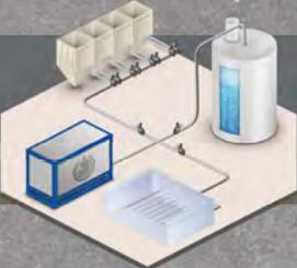
AGGREGATES AND WATER HEATING WITH ONE STEAM GENERATOR
