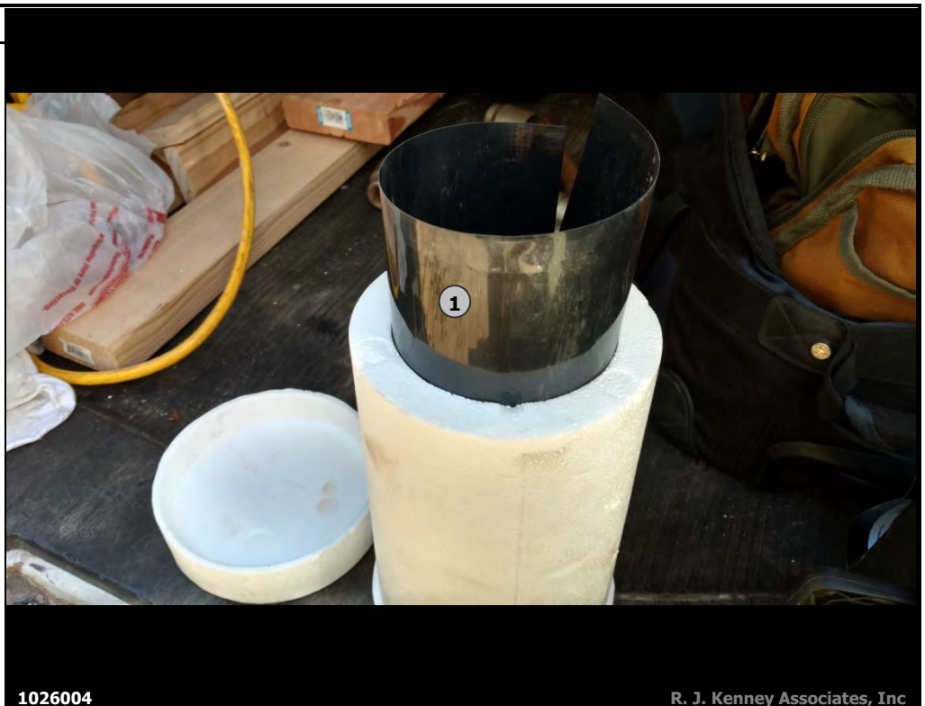
Cylinder Mold with HIPS Lining Partially Removed
