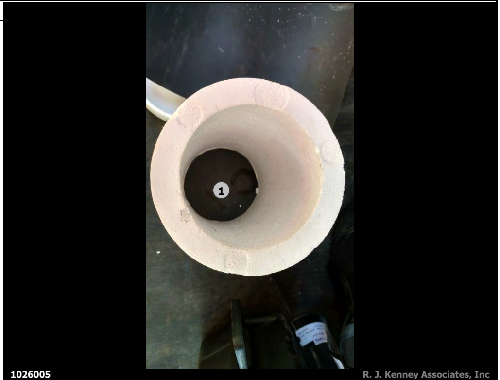
Top View of Typical Cylinder Mold Showing HIPS Lining at Bottom of Mold
